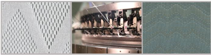
DOUBLE-KNIT ELECTRONIC JACQUARD MACHINE WITH 3 POSITION NEEDLE SELECTION.
